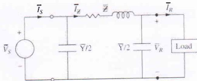
$$\begin{aligned} \text{The total line impedance } \bar{Z} &= (0.1826 + j0.784)100 = 18.26 + j78.4 \\ &= 80.5 \angle 76.89^\circ \Omega/\text{ph.} \end{aligned}$$
